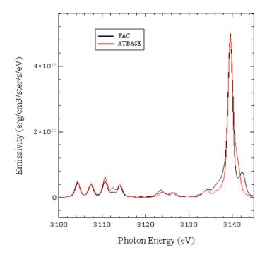
Simulation results for Ar-doped DD plasma at 600 eV temperature and 1 g/cc density computed with FAC and ATBASE data. Ar He-alpha transition and associated Li-like satellites.
